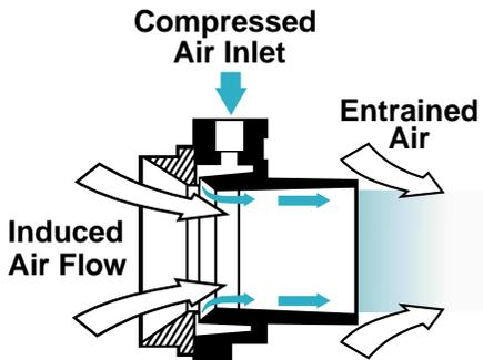
Transvectors use the impulse principle to achieve amplified airflows. When compressed air enters the Transvector, it fills a chamber that has only one exit path – a 0.002" (0.051mm) annular orifice. As the air is forced out of the orifice, it accelerates and collides with surrounding air entraining a great volume of free, ambient air. The result is a large volume of output air in return for a small amount of compressed air.
