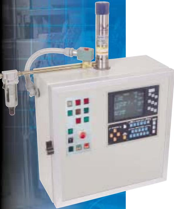
All Vortex Cooler systems include a 5-micron Auto-Drain filter and a ducting kit to distribute cold air throughout the enclosure. Thermostatically controlled models also contain a solenoid valve and thermostat, limiting compressed air usage to those times when cooling is required.
