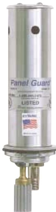
**Models 770 and 770-35H Panel Guard coolers** feature an integral, mechanical thermostat. A heat sensitive element at the base of the cooler activates a control valve to open/close the compressed air supply. The non-adjustable thermostat requires no electrical connections and will provide cooling protection to maintain enclosure temperatures in the range of 80-92°F (27-32°C).
