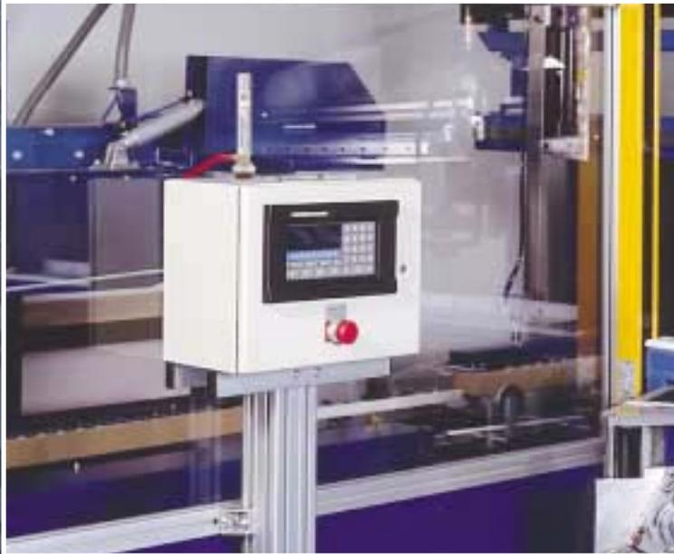
Have your production lines or equipment ever shutdown from overheated electrical enclosures? It's a common problem, and one that can have serious consequences. Research by control manufacturers has shown that for each 18°F (10°C) increase in temperature, online production shutdowns will occur twice as often. Vortex Coolers offer a simple, reliable and affordable solution to keeping control panels cool, clean and protected.
